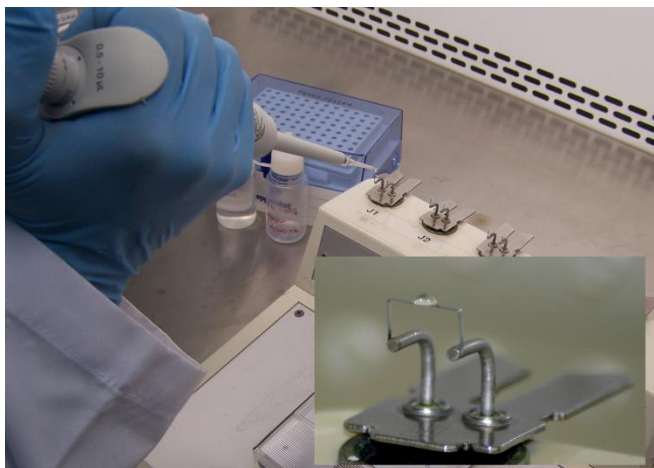
Figure 4. Loading of a sample on a filament
