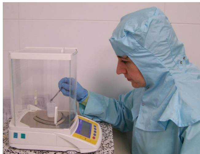
Figure 2. Weighing of a sample with an analytical balance
