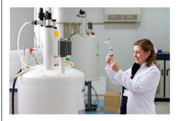
Nuclear Magnetic Resonance (NMR) is a spectroscopic technique which provides information about the structural and chemical properties of molecules. Using NMR, information about bonding structure and molecular formula can also be obtained.
