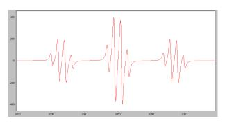
In ESR, spectrum is generated by obtaining the 'g' value by external microwave frequency is not changed but magnetic field frequency is changed.
