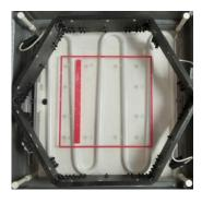
**2 Dimensional Gel Electrophoresis System (TDGE):** IEF and Vertical Electrophoresis systems are used sequentially to create a 2 dimensional gel image where Isoelectric Point (pl) and Molecular Weight of the proteins might be observed on a single gel. Samples in the range of nanograms/liter to miligrams/liter might be characterized by different staining techniques.
